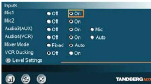
4. Adjust the audio Input Type Level if necessary (recommend +8dB)
