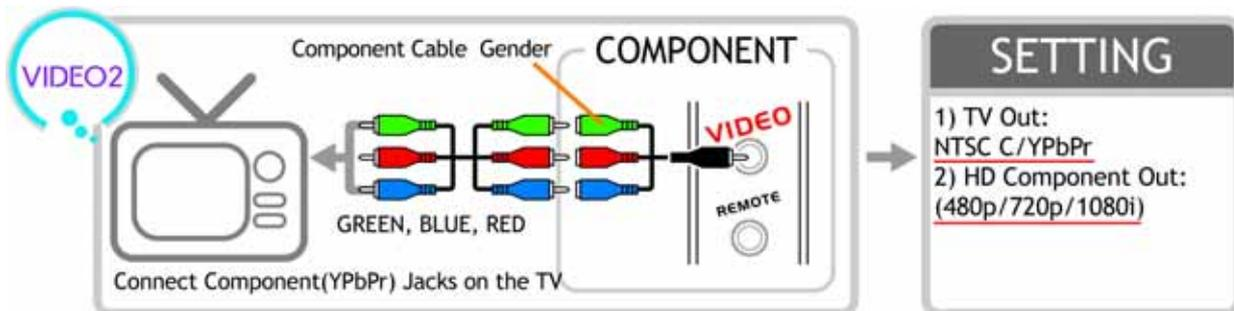
Connecting the Y(green), Pb(blue) and Pr(red) cable : HD component and Progressive Scan output are available and require a special type of cable and TV set.(Not supplied)
