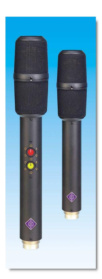
he SM 69 fet and USM 69 stereo microphones each have two separate dual-diaphragm capsules. These are mounted vertically and rotate against each other. The directional polar patterns can be selected separately for each capsule. The capsules operate independently from each other.
