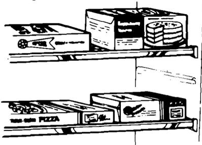
2. To speed freezing, lay packages in a single layer so each rests on the freezing surface of a shelf. Leave space between packages.
