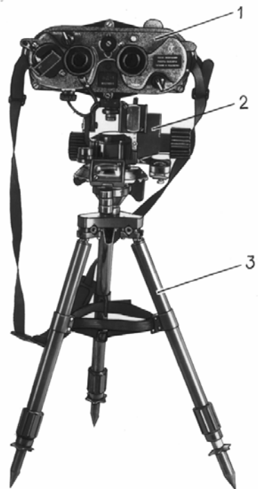
1 - Rangefinder; 2 - Angular Mount; 3 - Tripod
