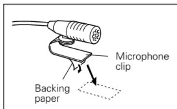
**2** Adjust the horizontal orientation of the microphone in such a way that it faces towards the driver.
