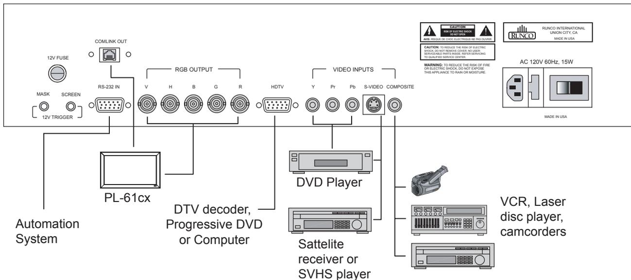
While there are many different ways to connect your source equipment to your PFP Controller, the examples shown above are the most common and are recommended by Runco.
