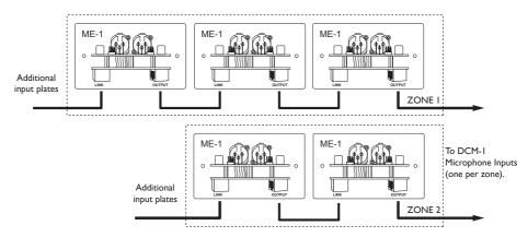
Note that it is not possible to intermix ME-Is with either Cloud LE-I or BE-I remote line input plates in this manner.
