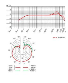
SpecificationsPolar patterncardioidFrequency range60 to 20,000 HzSensitivity4 mV/Pa (-52 dB
