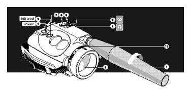
Set the preliminary focus adjustment by placing the adjusting mark (located on top of the objective focusing ring) opposite the letter "N" in the word "Normal" (11).
