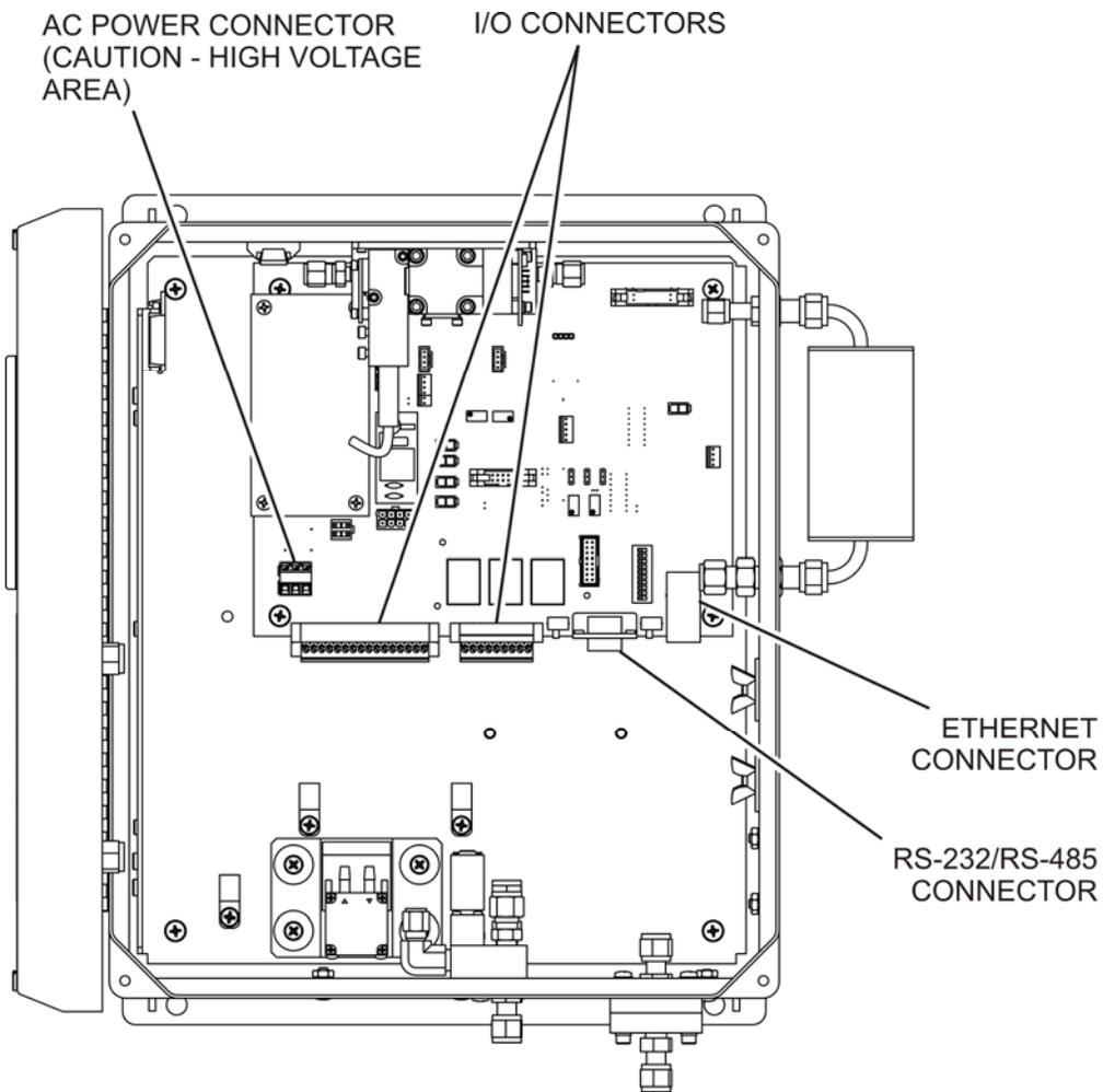
**Figure 4-6: NEMA Electrical I/O Connections**
