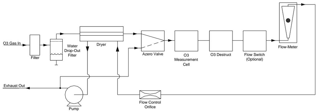
**Figure 10-2: Pneumatic Diagram (NEMA Version with Sample Conditioner)**
