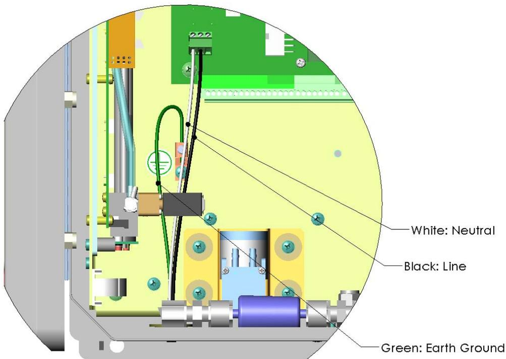
**Figure 4-2. NEMA AC Power Connection to Monitor**
