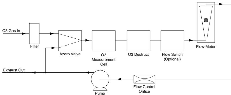
Figure 10-1: Pneumatic Diagram (Rack Mount Version)
