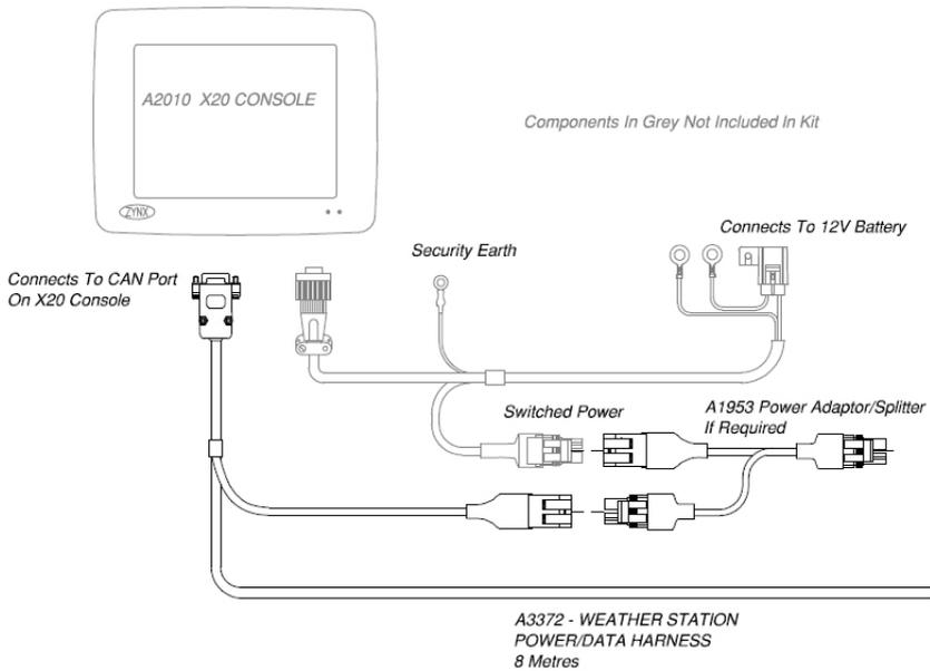
**Figure 5-2. In Cab Weather Station Layout**
