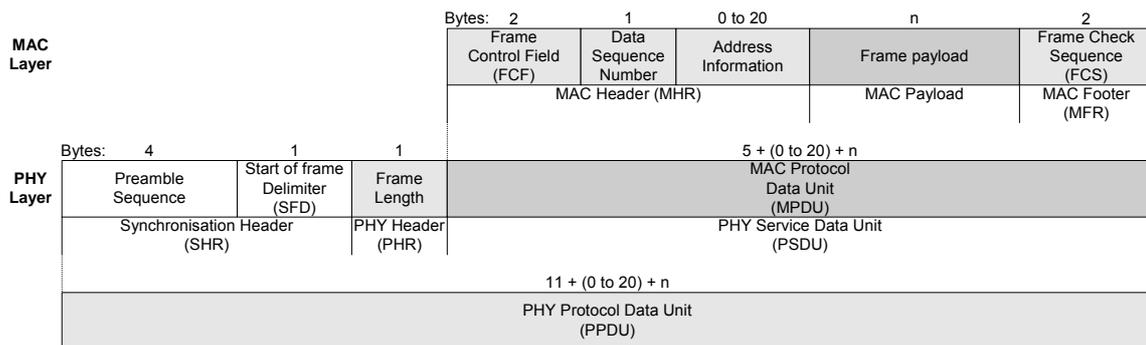
Figure 17. Schematic view of the IEEE 802.15.4 Frame Format [1]
