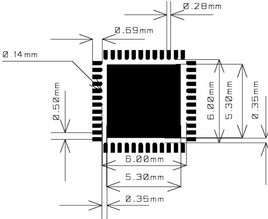
Note: The figure is an illustration only and not to scale. There are nine 14 mil diameter via holes distributed symmetrically in the ground pad under the package. See also the CC2420 EM reference design.
