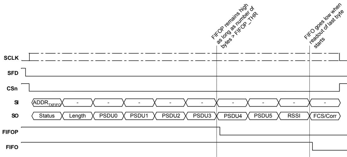
Figure 14. Example of pin activity when reading RXFIFO.
