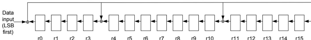
Figure 20. CC2420 Frame Check Sequence (FCS) hardware implementation [1]
