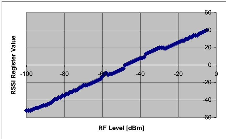
Figure 27. Typical RSSI value vs. input power
