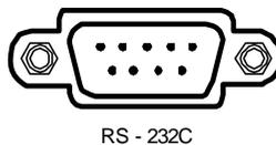
Use the RS232C port to connect an external modem for remote monitoring, configuration, and software upgrades, text input, and to connect a remote control keyboard. Use a modem cable with a DV9S (female) connector to connect to the DVR.
