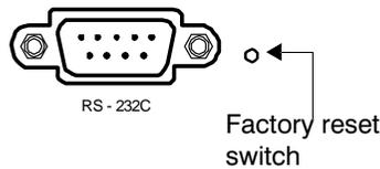
The DVR has a Factory Reset switch to the right of the RS232C connector. This switch will only be used on the rare occasions that you want to return all the settings to the original factory default settings.
