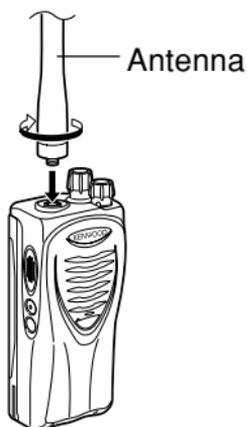
Screw the antenna into the connector on the top of the transceiver by holding the antenna at its base and turning it clockwise until secure.
