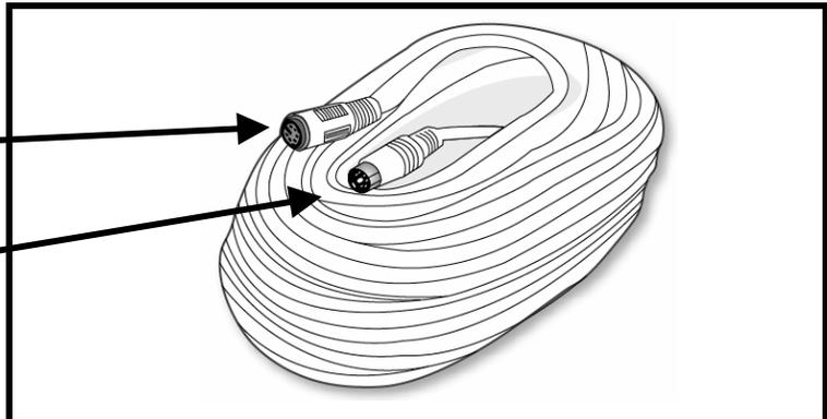
**6-PIN DIN FEMALE TO BNC MALE / RCA MALE COUPLER / FEMALE BARREL POWER CONNECTION**
