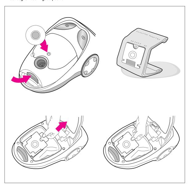
The Motor filter in the Dust bag compartment should be changed or washed when necessary. Wash the Motor filter with water and dry it out before using.
