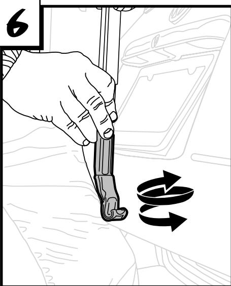
**• Rotate lower clamp arm until edge of clamp just clears bottom edge of hatch.**
