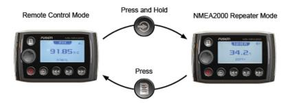
The NRX200 remote control can be configured to display NMEA2000 network data, the following options are available:
