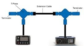
**NOTE**: The supplied Terminators must be fitted to the ends of the network as shown. Failure to do so will affect operation.
