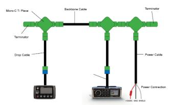
**Note:** The supplied Terminator must be fitted to the ends of the network as shown. Failure to do so will effect operation.
