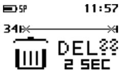
An x symbol appears at the beginning and the end of the file to indicate that the sound file is marked to be deleted.
