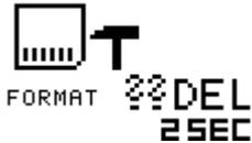
To reconfirm and start the reformatting process, press the DEL button for at least 2 seconds. This will erase all data on the memory card permanently.
