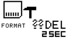
To confirm and start the formatting process, press the DEL button for at least 2 seconds. If you want to cancel the formatting process, either remove the memory card or move the 4-Position Switch.
