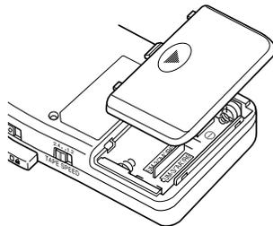
2. Insert the batteries into the compartment as indicated by the polarity symbols (+ and -) marked inside.
