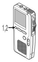
Select any file in the folder, then press and hold the **ERASE** button for 3 seconds or longer.
