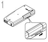
Slide the card cover lock in the direction indicated by the arrow.
