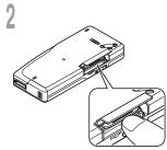
Push the card inward to unlock it, and let it eject partially.
