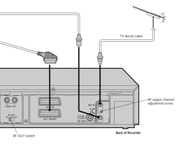
The video recorder sends picture and sound signals via the RF connecting cable to your TV on UHF channel 36.
