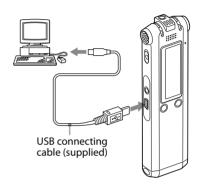
While the batteries are charging, "CONNECTING" and the battery indicator are displayed in an animation.
