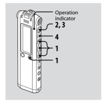
When "ADD/OVER" in the menu is set to "ADD," you can add a recording to the message being played back. The added recording will be placed after the current message, and will be counted as a part of the message.
