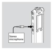
1 Connect an external microphone to the \(^\circ\) (microphone) jack when the IC recorder is in the stop mode.
