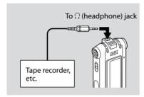
To record the sound of the IC recorder with other equipment, connect the  $\Omega$  (headphone) jack of the IC recorder to the audio input connector (minijack, stereo) of other equipment using an audio connecting cable\*.
