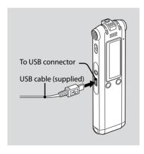
You can charge the rechargeable batteries by connecting the IC recorder to an AC outlet using a USB AC adaptor (not supplied).
