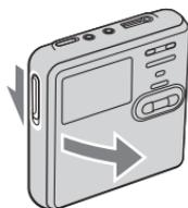
2 Insert a disc with the label side facing front, and press the lid down to close.
