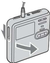
2 Insert a disc with the label side facing front, and press the lid down to close.
