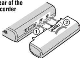
2 Insert a LR6 (size AA) alkaline dry battery. Inset the battery
