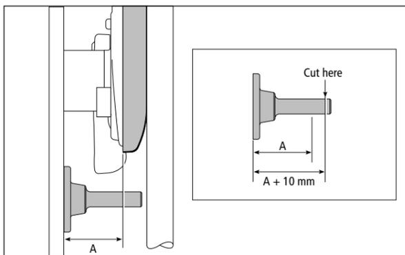
2. Use a hacksaw to cut the pin **10 mm (0.4 in) LONGER** than dimension A. Remove any sharp edges with a file or sandpaper.
