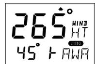
**Note!** The apparent wind speed must be more than 3 knots. If the apparent wind speed falls below 3 knots, wind signals are disabled and the Autopilot will maintain the current magnetic heading reference instead.
