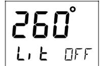
To select between the 4 light levels [LOW], [MID], [MAX] and [OFF], press **RIGHT**. To lock the selected level, press **SET**.
