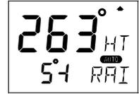
To activate power steering, press **SET** when [RAI] is flashing. The rudder angle, followed by a sign for port or starboard is displayed on the lower-line.
