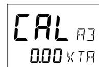
If the pilot's cross track error exceeds the set threshold of distance of the track, the alarm will be activated.
