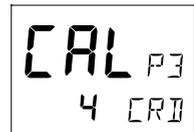
Course holding with heavy and difficult to steer boats, is greatly improved, when using this feature. Too little counter rudder, will allow the boat to overshoot on large course changes. Too much will cause unnecessary rudder corrections and a tendency to stop short of coming to a new course, requiring several successive corrections before easing up to the new heading.
