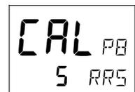
The [RRS] will be set to [5] after the APC routine is performed. It is then possible to increase or decrease the speed reduction of the pumpset motor.
