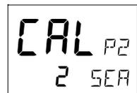
Damping of wind transducer. The factory default setting should be adequate. In very heavy weather or unstable wind conditions, unnecessary corrections may be minimised by increasing the setting.
