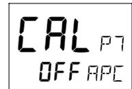
The Autopilot will not function unless the boat pass the APC routine. The APC will automatically determine and correct how wires and pipes are connected. It will also learn how the boat reacts on different rudder commands and automatically calibrate itself.
