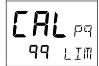
The rudder angle limit sets maximum angle for the rudder. If the limit is set to 45°, it is not possible to exceed a rudder angle 45° on either port or starboard. Check the maximum rudder angle by turning the steering wheel to port and starboard and read the maximum angle. If the angle is greater on one side, decrease the smallest angle by 3°, and enter that setting as the limit.
