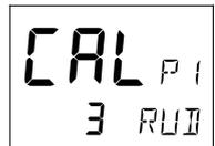
The rudder should be set to the position where positive control of the steered course desired, is achieved without undue activity. Run the boat at its cruising speed and make a course change of 40°, with the push buttons. The boat should not overshoot by more than approximately 5°. Adjust the rudder until this is achieved.
