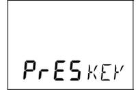
To initialise the instrument, press **SET**, **one instrument at a time**, on all installed digital instruments,.
