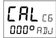
To check the transducer position, sail/steer your boat in a straight line towards two visible objects in a line. If the actual heading taken from the sea chart is 330° and the compass displays 335°, then set the value of 360° - 5° to 355°.
