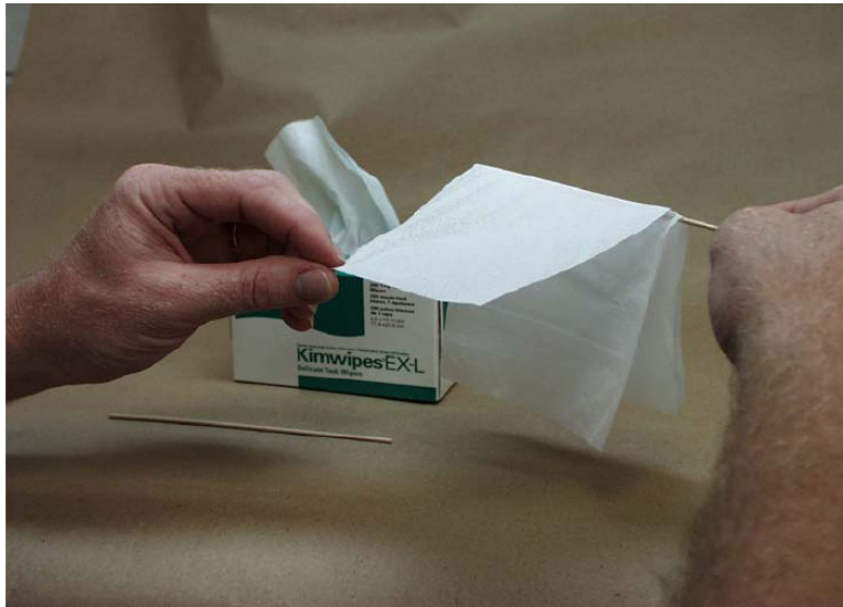
Figure 6-2. Preparations for Cleaning the Low Range Cylinder
