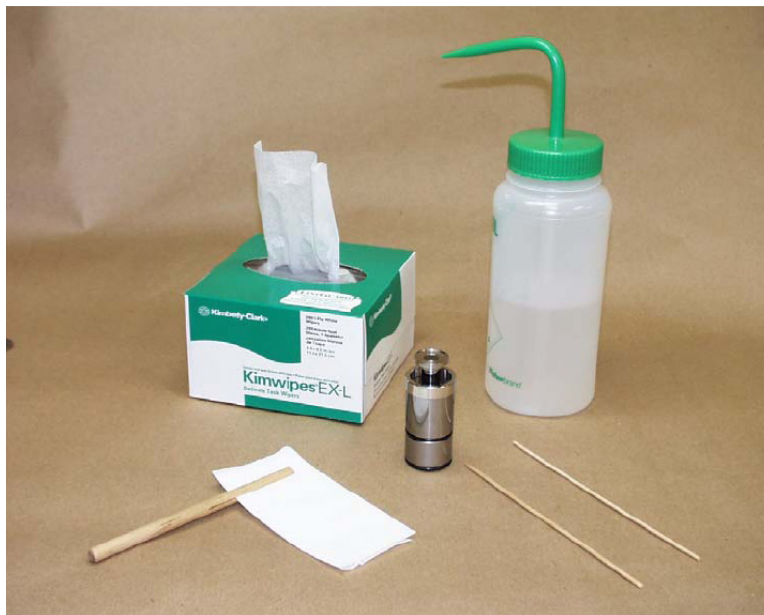
Figure 6-7. Materials for Cleaning the Mid Range Piston/Cylinder
