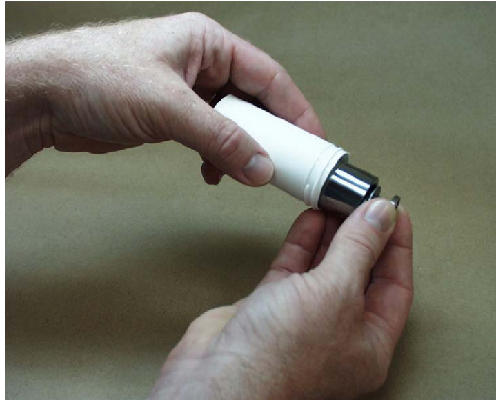
Figure 5-4. Removing Low Range Piston and Cylinder from Container - Step 2
