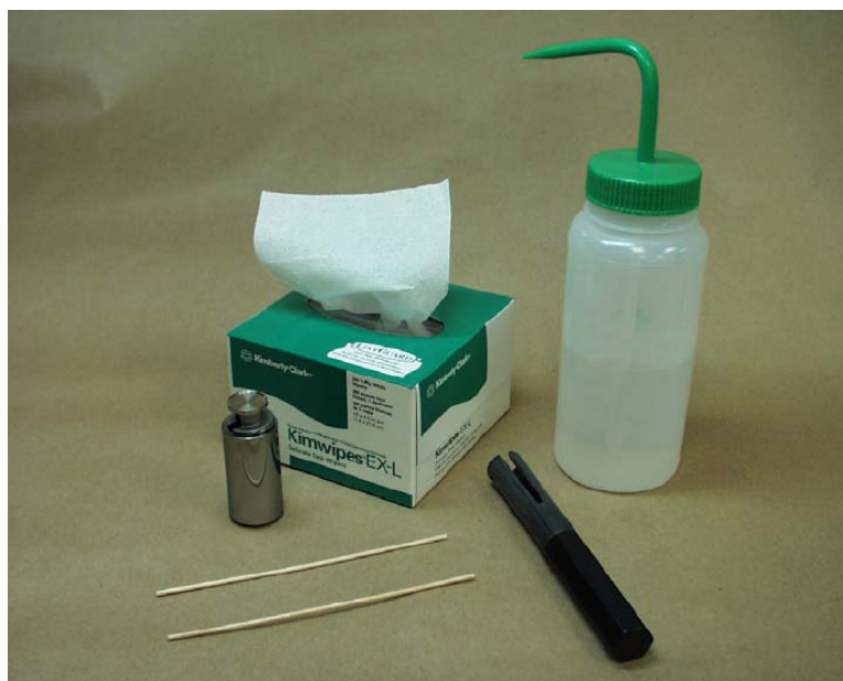
Figure 6-1. Materials for Cleaning Low Range Piston/Cylinder
