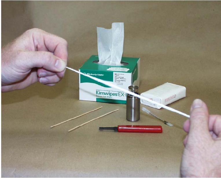
Figure 6-12. Preparing the Kim Wipe for Cleaning the High Range Cylinder - Step 3
