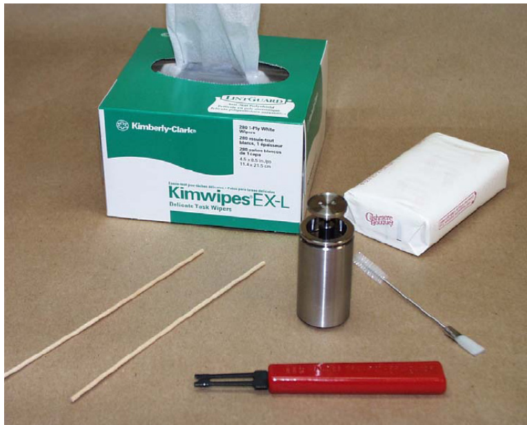
Figure 6-9. Materials for Cleaning the High Range Piston Cylinder
