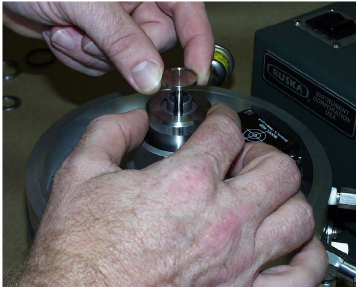
Figure 5-7. Positioning the Upper Thrust Washer/Piston Retainer in the Cylinder Retaining Cap Recess
