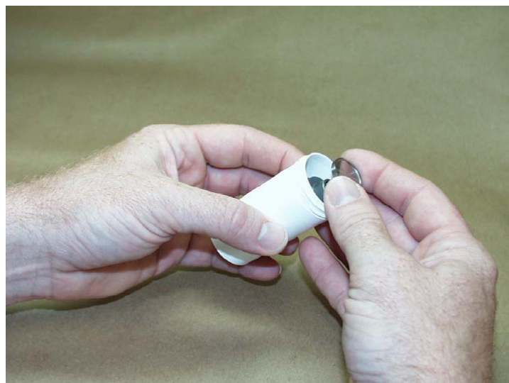
Figure 5-3. Removing Low Range Piston and Cylinder from Container - Step 1
