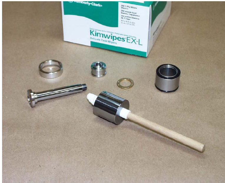
Figure 6-8. Preparing the Mid Range Cleaning Tool
