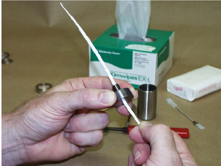
Figure 6-14. Drying the High Range Cylinder
