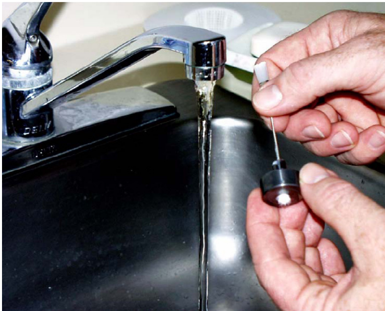
Figure 6-13. Cleaning the High Range Cylinder
