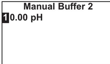
12. Watch the pH reading for sensor 2 (**S2**) at the top of the screen. Once the reading is stable, enter the pH value of the buffer at the buffer temperature and press ENTER.
