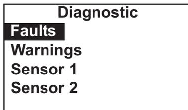
1. To read diagnostic messages, press DIAG. The screen at left appears. To display fault messages, select **Fault**. To display **Warning** messages select warning. To read measurement information about the sensor(s) including raw sensor signal and calibration data, choose the desired sensor and press ENTER.
