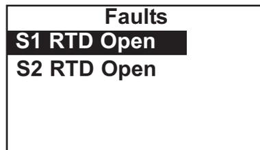
2. If you choose **Fault** or **Warning**, a screen like the one shown at left appears. **S1** means sensor 1. **S2** means sensor 2. For additional troubleshooting information, select the desired message and press ENTER. For more information, see Section 9.3.
