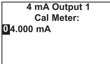
4. The analyzer will simulate the low output current. Change the value in the display to match the reading from the milliammeter.
