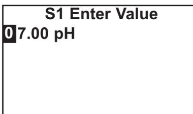
7. Once reading is stable, measure the pH of the liquid using a referee instrument. Because the pH of many natural and treated waters depends on temperature, measure the pH of the sample immediately after taking it. For poorly buffered samples determine the pH of a continuously flowing sample from a point as close as possible to the sensor.
