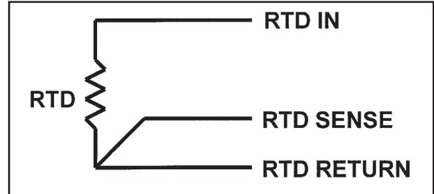
FIGURE 9-5. Three-Wire RTD Configuration.
