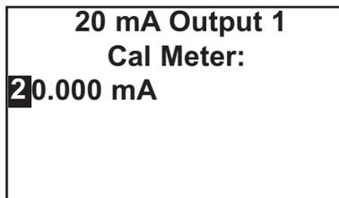
5. The analyzer will simulate the 20 mA output current. Change the value in the display to match the reading from the milliammeter.
