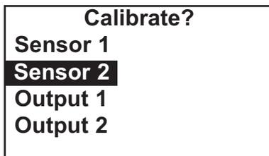
4. Choose the sensor you wish to calibrate. **Sensor 1** is the chlorine sensor. **Sensor 2** is the pH sensor.
