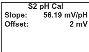
8. If the calibration is successful, the screen at left will be displayed for five seconds. The display will then return to screen in step 3.
