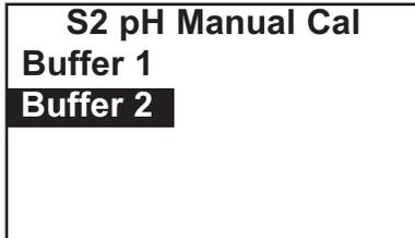
11. The display returns to the screen shown in step 8. Choose **Buffer 2**. Remove the sensor from the first buffer. Rinse with water and place it in the second buffer. Be sure the glass bulb and reference junction are completely submerged. Swirl the sensor. Press ENTER.
