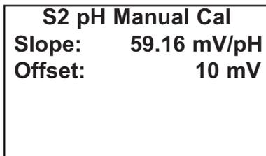
13. If the calibration is successful, the screen at left will be displayed for five seconds. The display will then return to screen in step 6.
