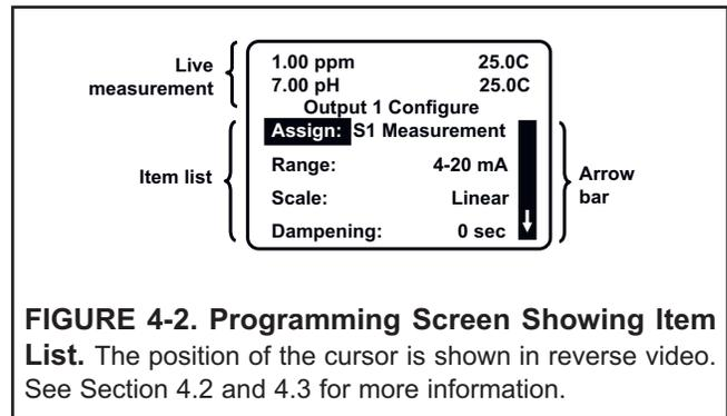
FIGURE 4-2. Programming Screen Showing Item List. The position of the cursor is shown in reverse video. See Section 4.2 and 4.3 for more information.
