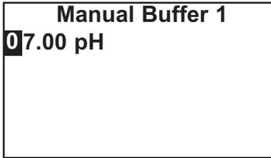
10. Watch the pH reading for sensor 2 (**S2**) at the top of the screen. Once the reading is stable, enter the pH value of the buffer at the buffer temperature and press ENTER.
