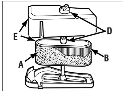
Figure 5-3: Briggs and Stratton air cleaner assembly.
