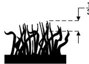
Cutting more than 1/3 of grass length may cause the grass to become excessively dry. In tall grass, it may be necessary to mow at a higher setting and then mow again at the desired height. NOTE: The cutting height is critical to achieving a well-groomed lawn. You should experiment with various settings to find that “just right” cutting height.
