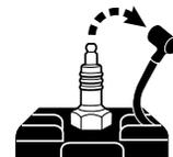
12. Shut the engine off, wait until the blade comes to a complete stop, and disconnect the spark plug wire before installing or removing the mulcher cover or the optional grass catcher. Make certain that the grass catcher is securely attached before operating the mower. Empty the grass catcher after each use—decomposing debris could generate enough heat to catch fire.
