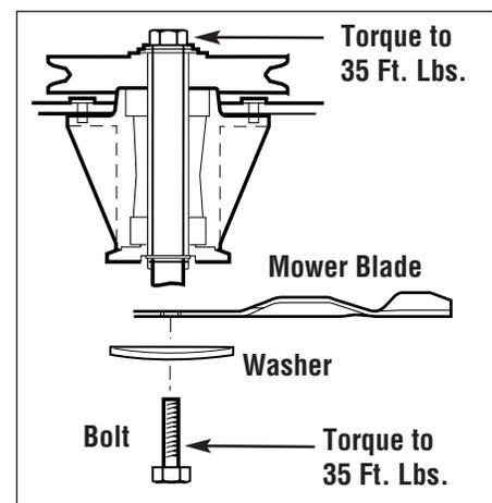
Figure 5-18: Blade spindle.
