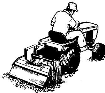
36" TILLER - Powered by tractor PTO.
