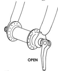
**⚠ WARNING:** The full force of the cam action is needed to clamp the wheel securely. Holding the nut with one hand and turning the lever like a wing nut with the other hand until everything is as tight as you can get it will not clamp the wheel safely in the dropouts.
