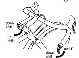
**▲ CAUTION: Never move the shifter while pedaling backward, nor pedal backwards after having moved the shifter. This could jam the chain and cause serious damage to the bicycle.**
