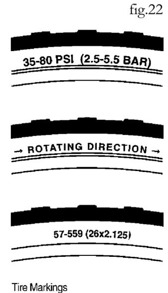
**⚠ WARNING:** Never inflate a tire beyond the maximum pressure marked on the tire's sidewall. Exceeding the recommended maximum pressure may blow the tire off the rim, which could cause damage to the bike and injury to the rider and bystanders.
