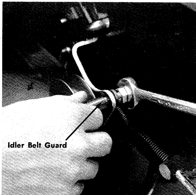
FIGURE 16. IDLER BELT GUARD
