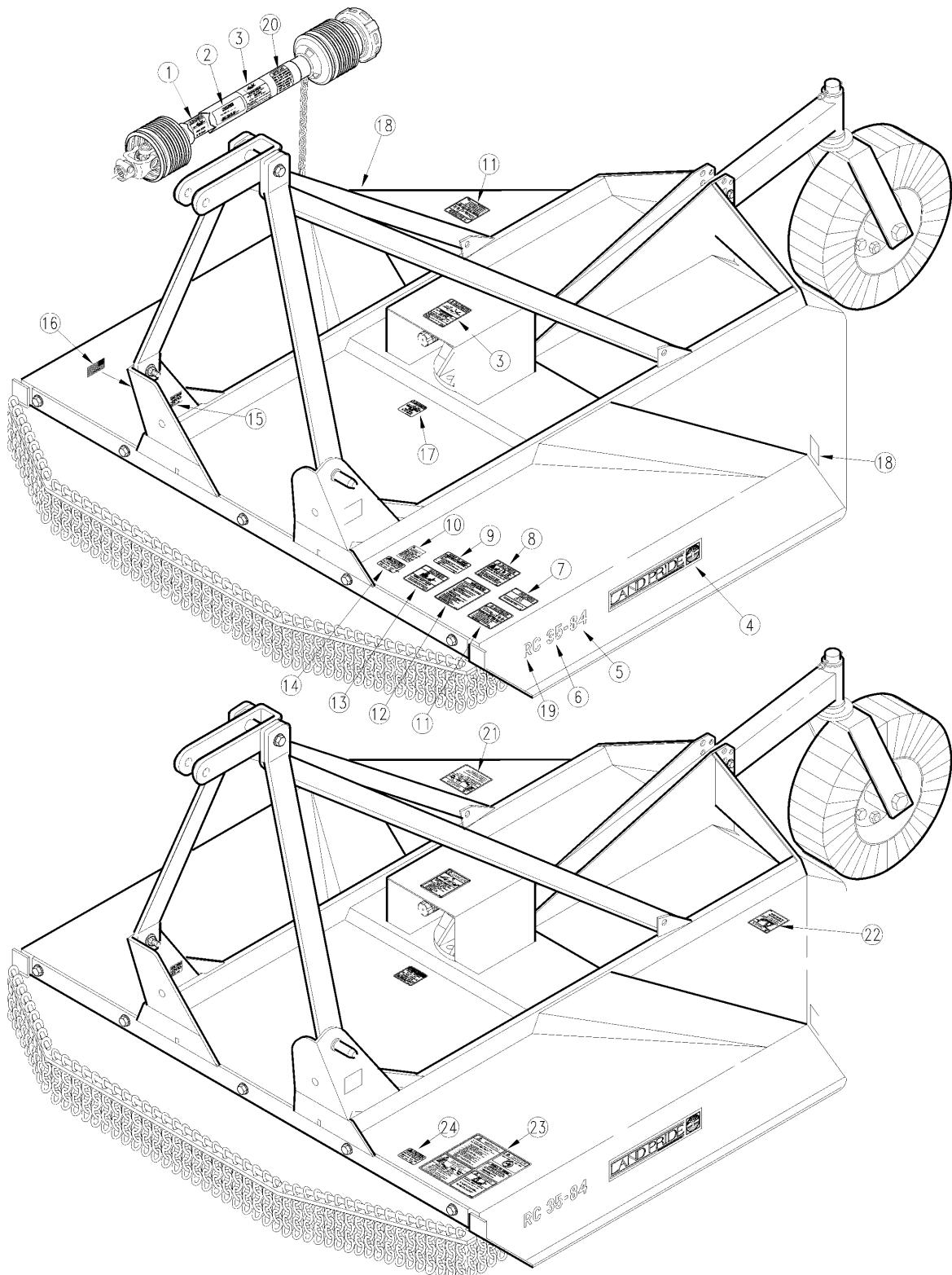
***Label Placement*****Applies to RC3560, RC3572, RC3584**
