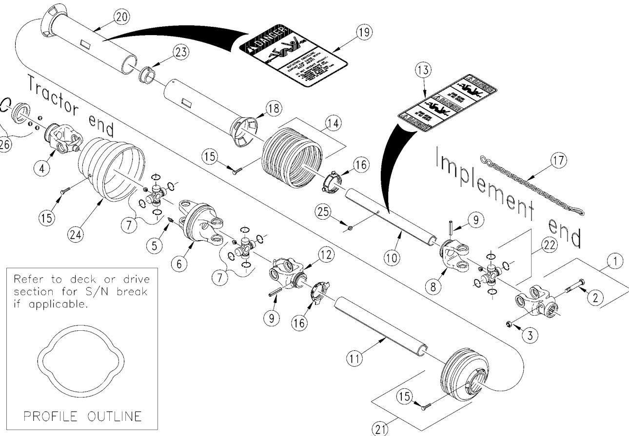
***Driveline CV Pull Type Cutter 1000 RPM (826-063C) Walterscheid*****Applies to RCM35120**
