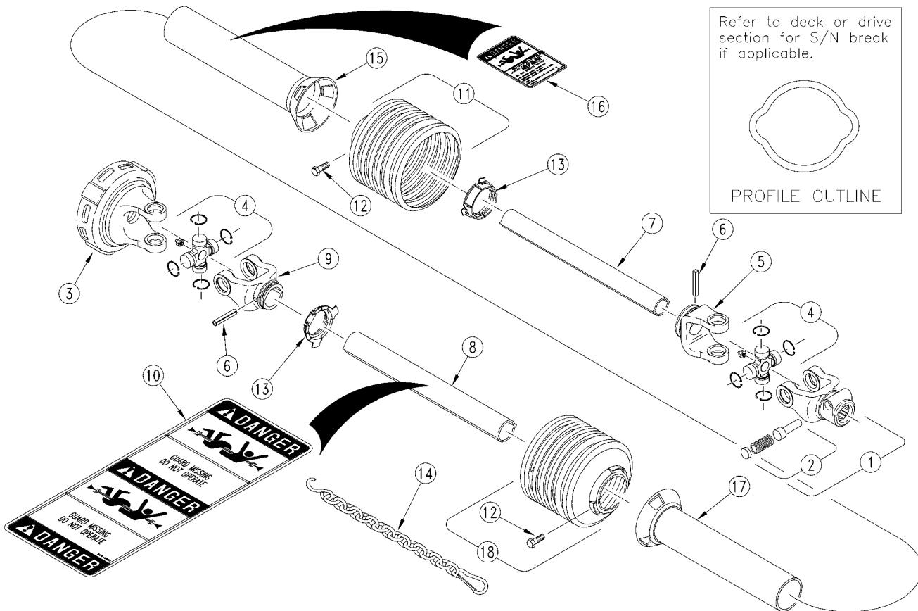
***Driveline Lift Type Cutter 1000 RPM (826-061C) Walterscheid*****Applies to RCM35120**
