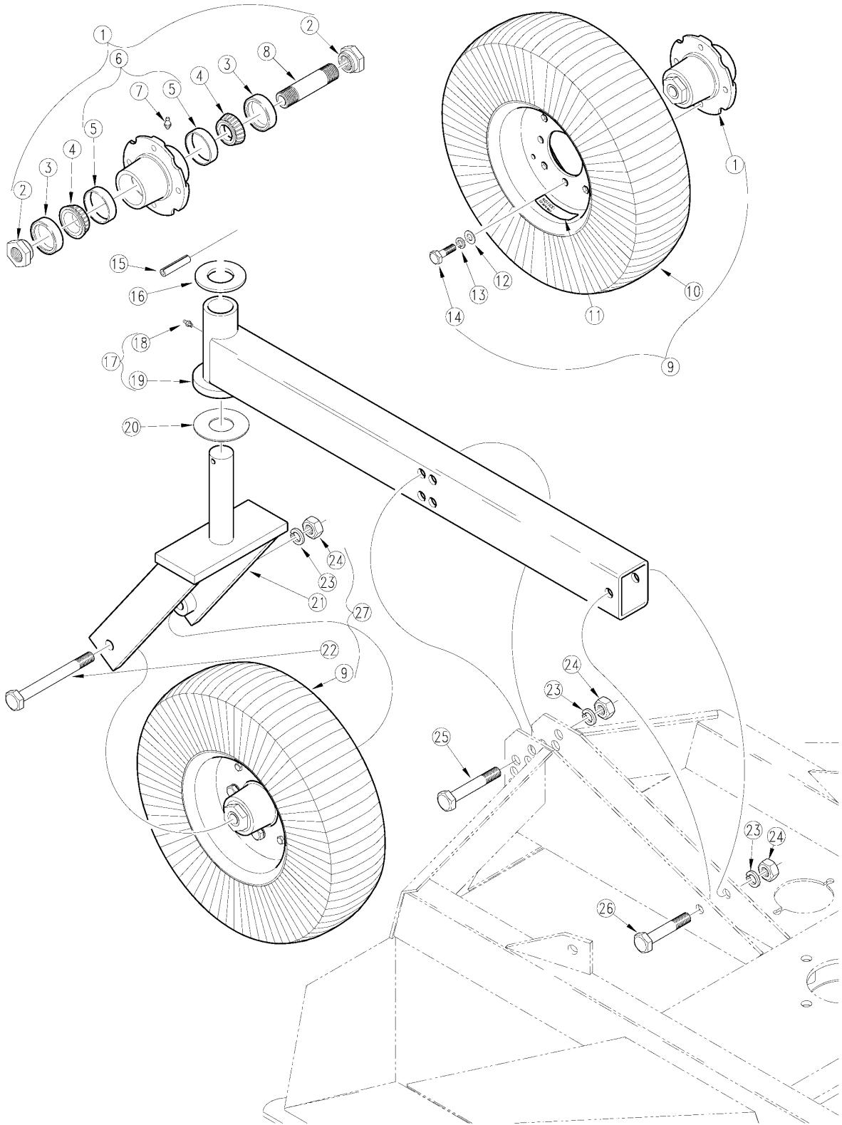
**Tailwheel****Applies to RC3560, RC3572, RC3584**
