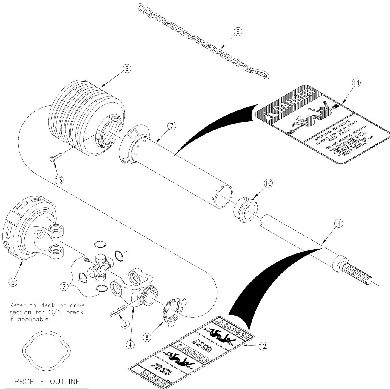
***Driveline Pull Type 1000 RPM (826-062C) Walterscheid*****Applies to RCM35120**
