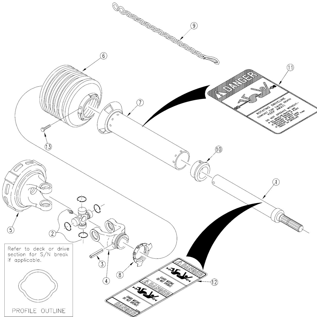
***Driveline Pull Type 540 RPM (826-052C) Walterscheid*****Applies to RC35120**
