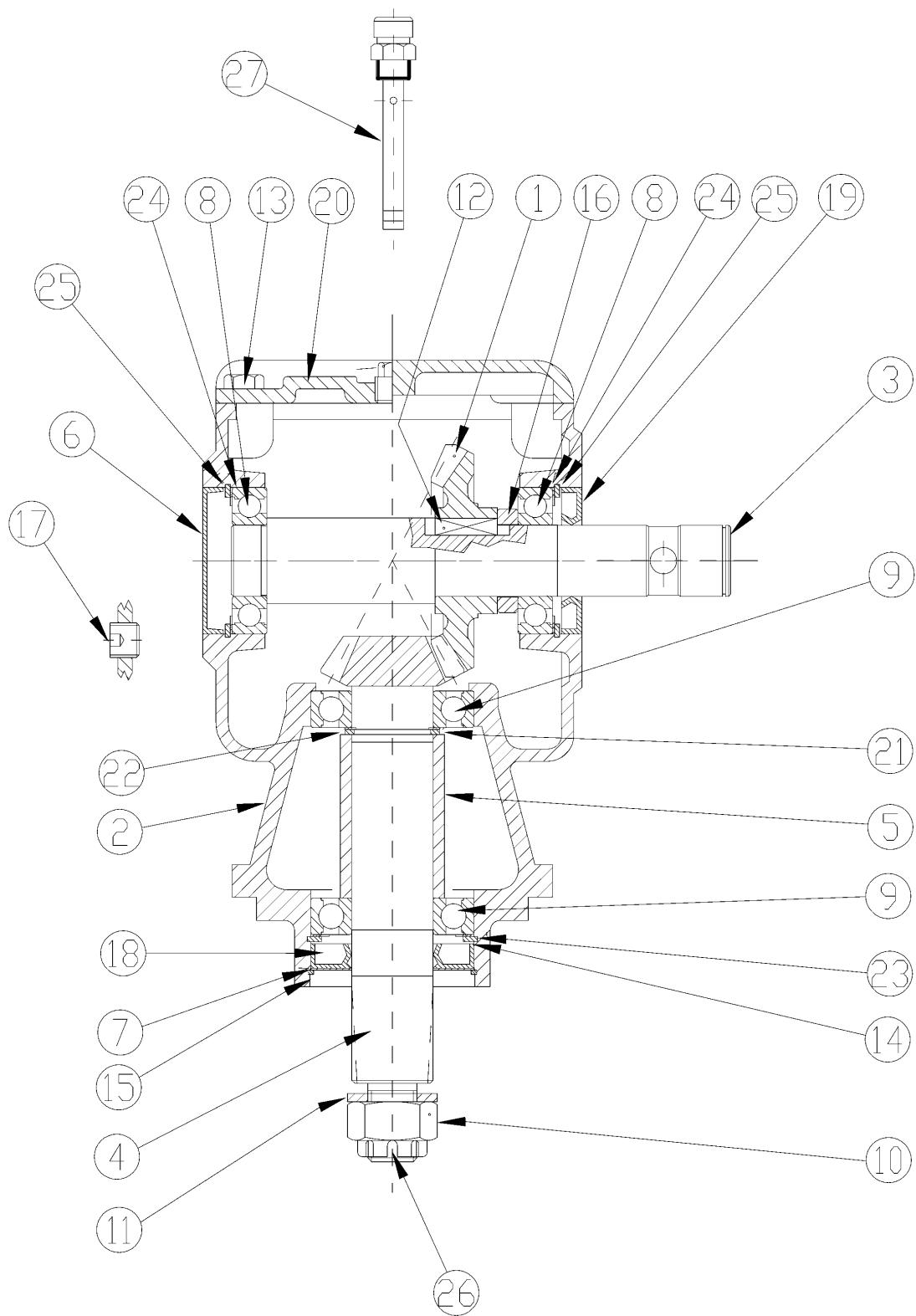
**Gearbox (826-383C) Comer (Service Only)****Applies to RC1548, RC1560, RC1572**
