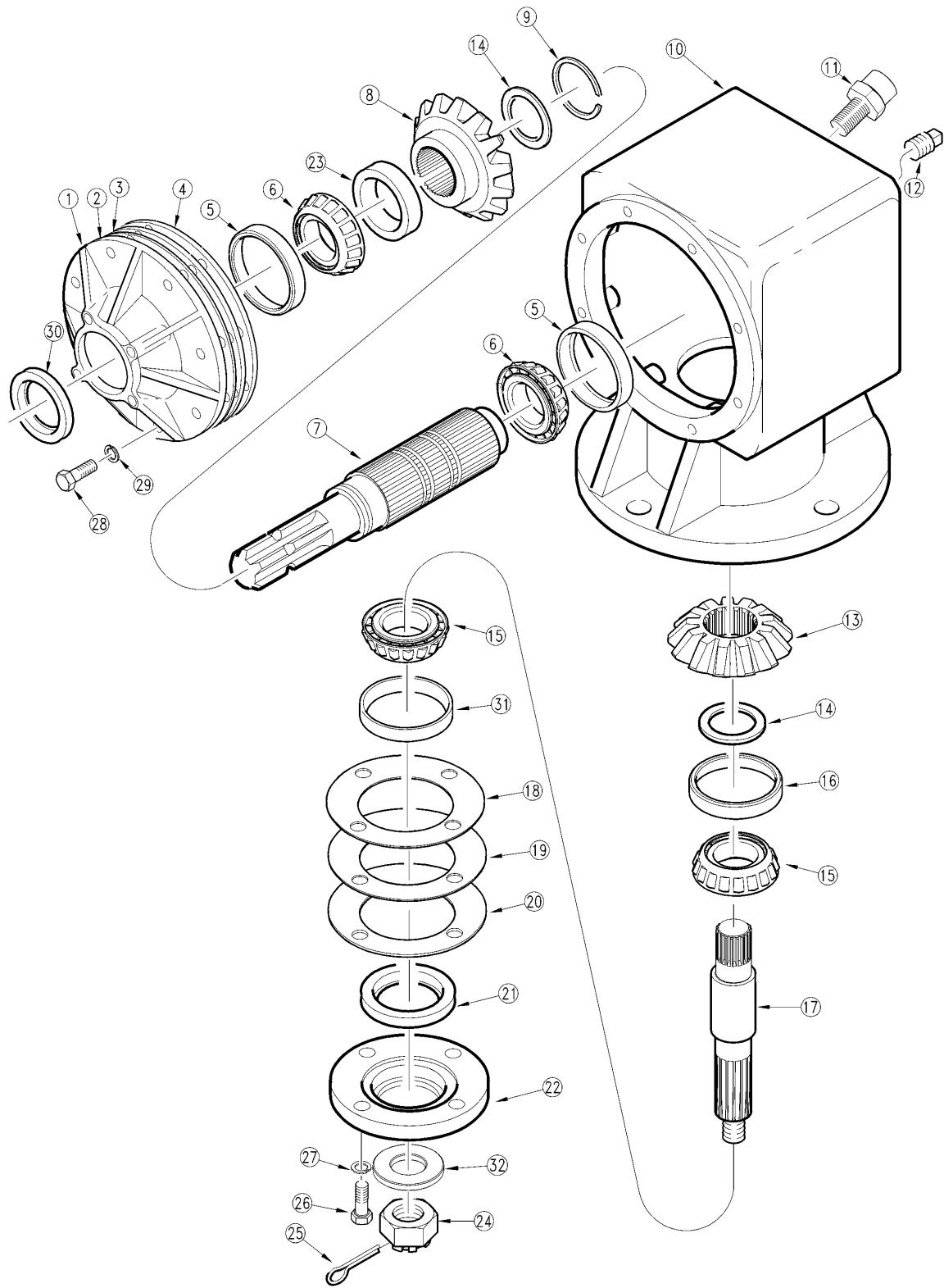
**Gearbox 540 RPM (826-035C) OMNI****Applies to RC35120**
