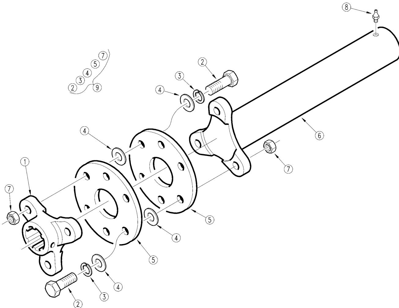
***Driveline Flex Coupler Shaft (826-054C)*****Applies to RC35120, RCM35120**
