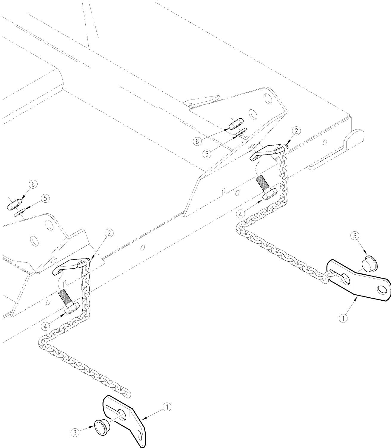
**Check Chain Kit****Applies to RC3560, RC3572, RC3584**
