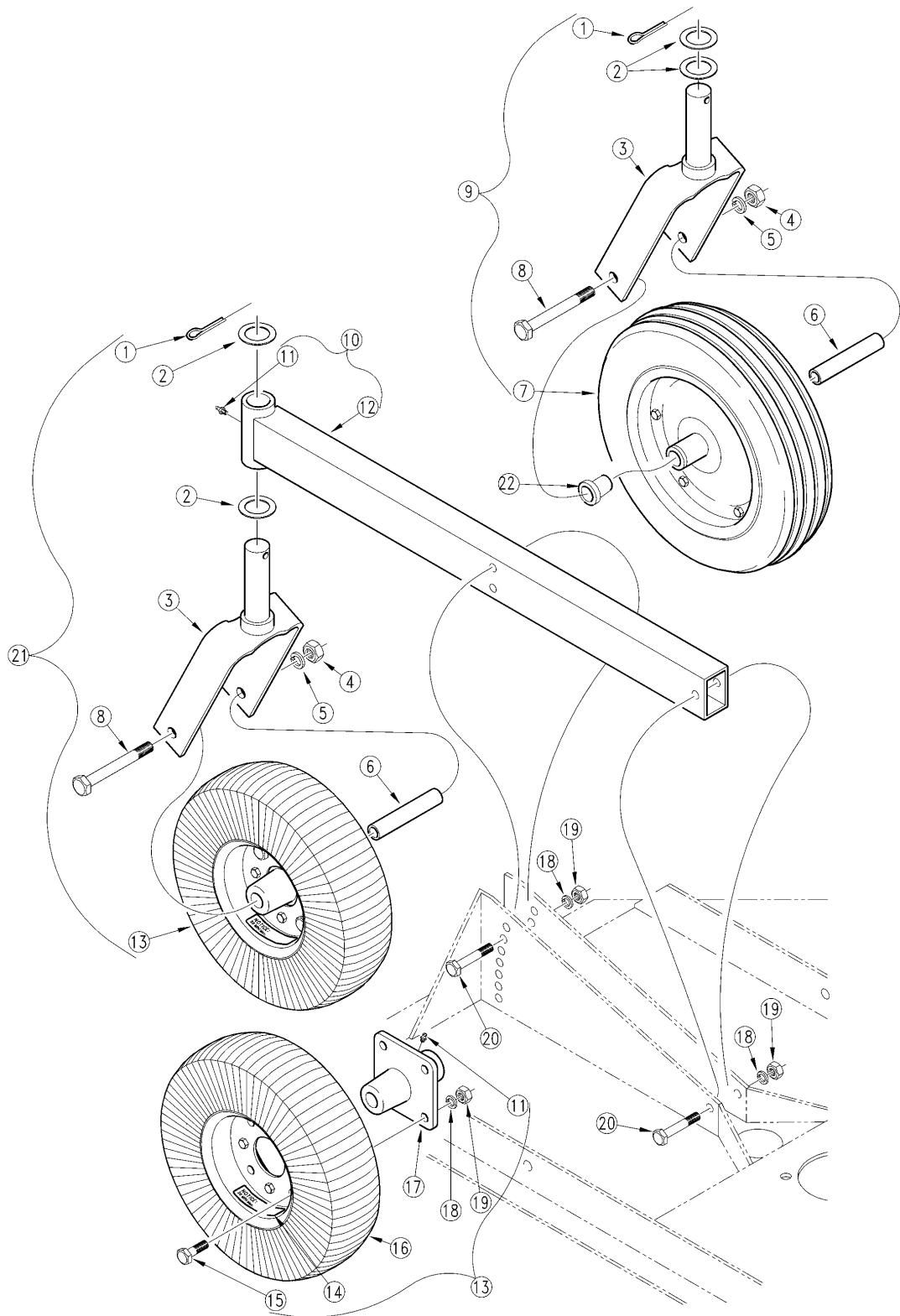
**Tailwheel****Applies to RC1548, RC1560, RC1572**
