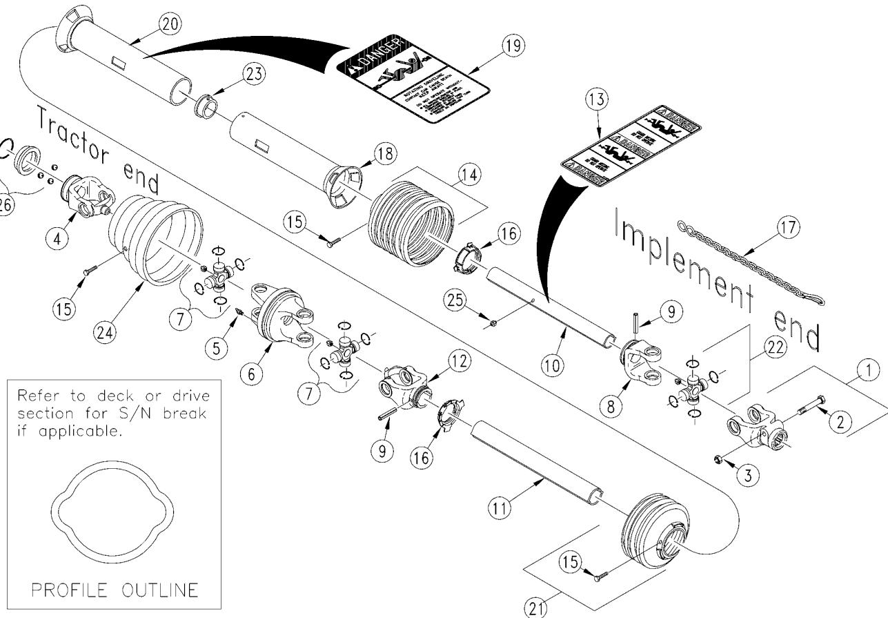
***Driveline CV Pull Type Cutter 540 RPM (826-053C) Walterscheid*****Applies to RC35120**
