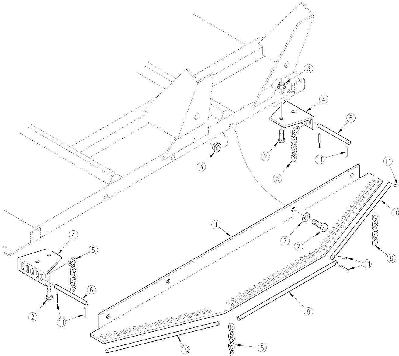
***Guard Front Safety Chain*****Applies to RC2560, RC2572, RC2584**
