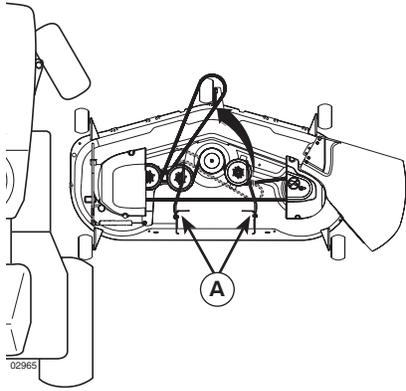
**NOTE:** Be sure mower side suspension arms (A) are pointing forward before sliding mower under tractor.
