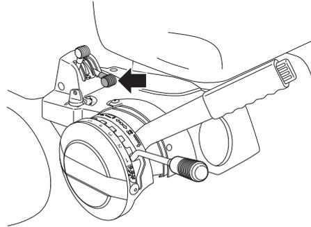
For cold starting the lever is moved backwards to its end position.
