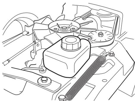
**Rider 15T** Fill if necessary with engine oil SAE 10W/40 (class SF-CC).
