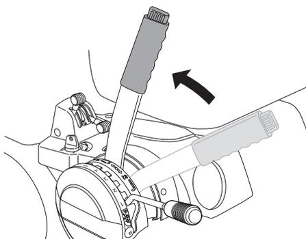
If the lock button is pressed in and the lever is moved forwards the unit will be lowered and the blades will automatically start to rotate (mowing position).
