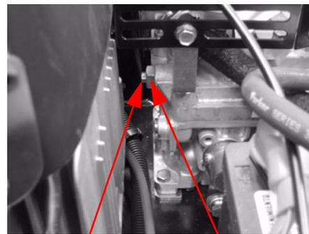
Inner bolt, 8mm      Jam Nut, 15mm
