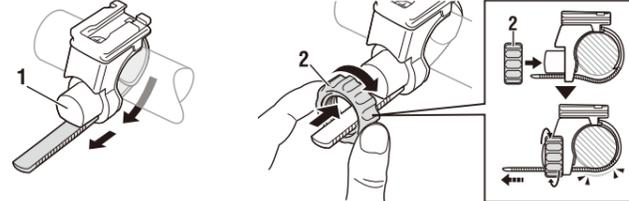
When cutting off the protruding part of the bracket band, round the edges to prevent injuries.
