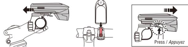
When using this light, always make sure to slide the light onto the bracket completely (until it "clicks" into place). Please be sure to securely attach the light to your bicycle. If it becomes loose, it may be dangerous.
