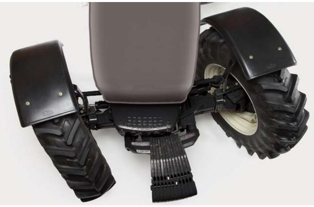
All Genesis FWD models are available with an optional Ultrasteer<sup>®</sup> front axle for a sharper turning radius that increases productivity. Tighter turning yields better fuel efficiency and reduces time wasting maneuvers. Add the optional traction control system (TCS), with front differential locks to make this tractor a real workhorse in the field. All TCS models can be ordered with optional front duals for increased traction and flotation.
