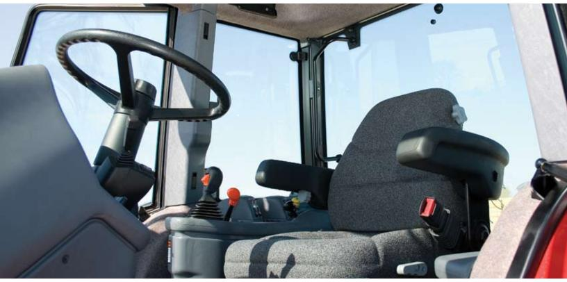
The Genesis combines operator comfort and function. Two doors access the clean, quiet and ergonomically correct cab interior. The cab is designed for excellent visibility to all interior and exterior tractor functions.
