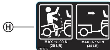
H. Weight Limitation. Notes limits of weight when towing implements. Refer to Operation section.
