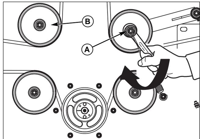
**Figure 46. Mower PTO Belt (72" Mower Deck)**
