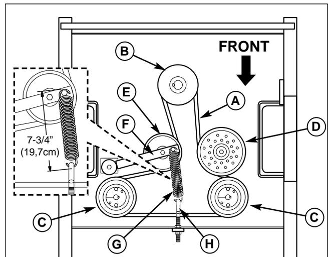
**Figure 44. Hydraulic Pump Drive Belt Replacement**
