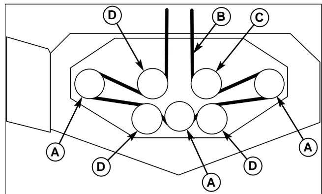
**Figure 47. Mower PTO Belt Routing**
