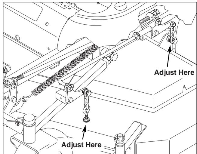
**Figure 42. Deck Level & Spring Length Adjustment**
