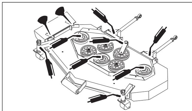
Figure 18. Deck Lubrication
