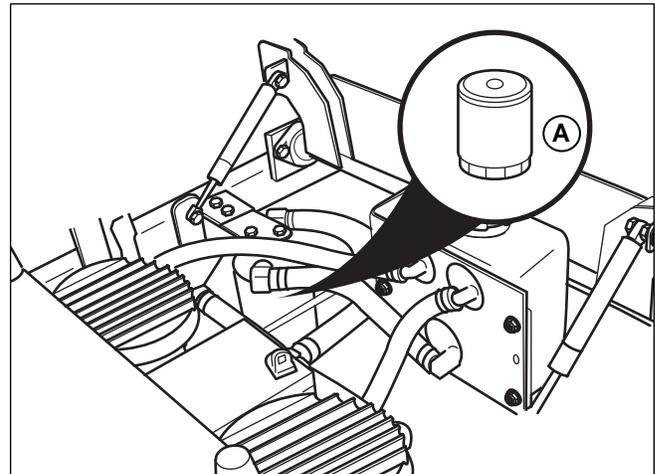
**Figure 14. Hydraulic Oil Filter Location**
