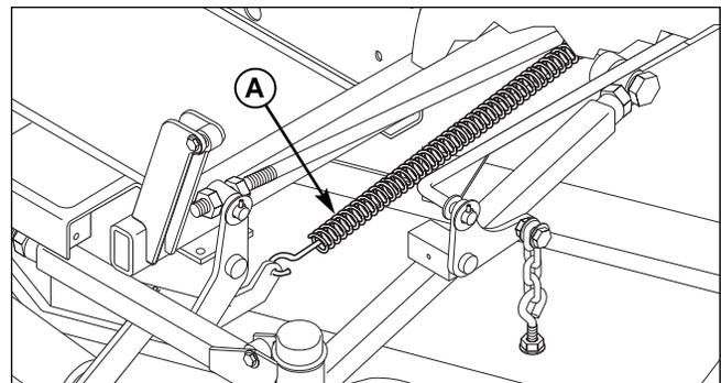
**Figure 43. Deck Lift Spring Location
