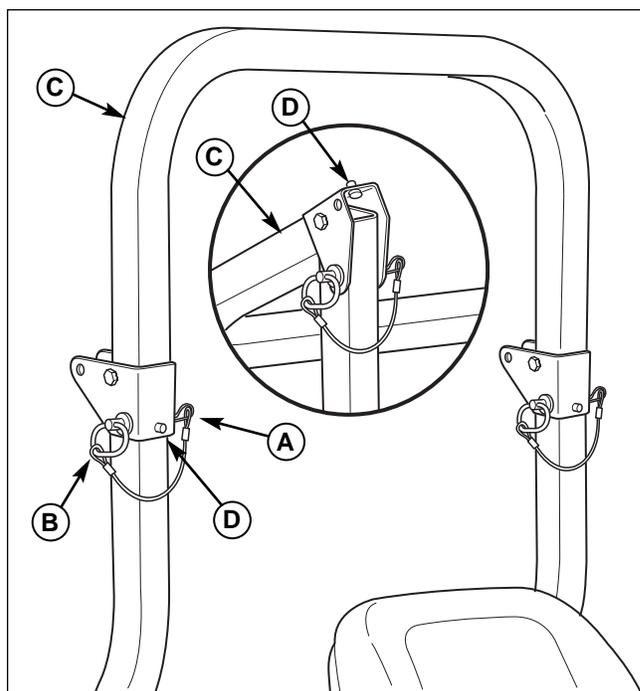
**Figure 10. Raise & Lower the Roll Bar**
