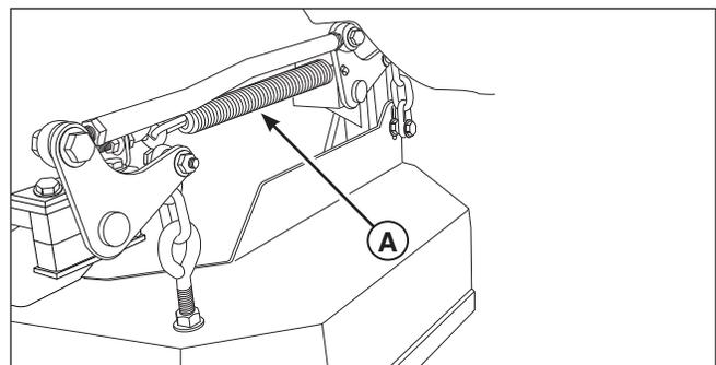
Figure 43. Deck Lift Assist Springs Location
