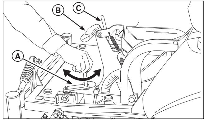
Figure 36. Mowing Height Adjustment
