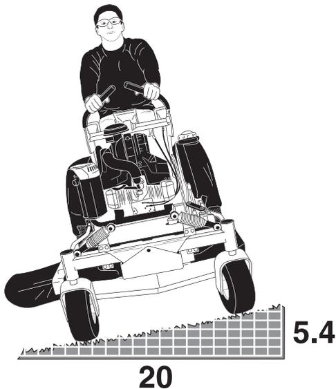
Operation on slopes can be dangerous. Using the unit on a slope that is too steep where you do not have adequate wheel traction (and control) can cause sliding, loss of steering, control, and possible rollover. You should not operate on a slope greater than a 5.4 foot rise over a 20 foot length (15 degrees).
