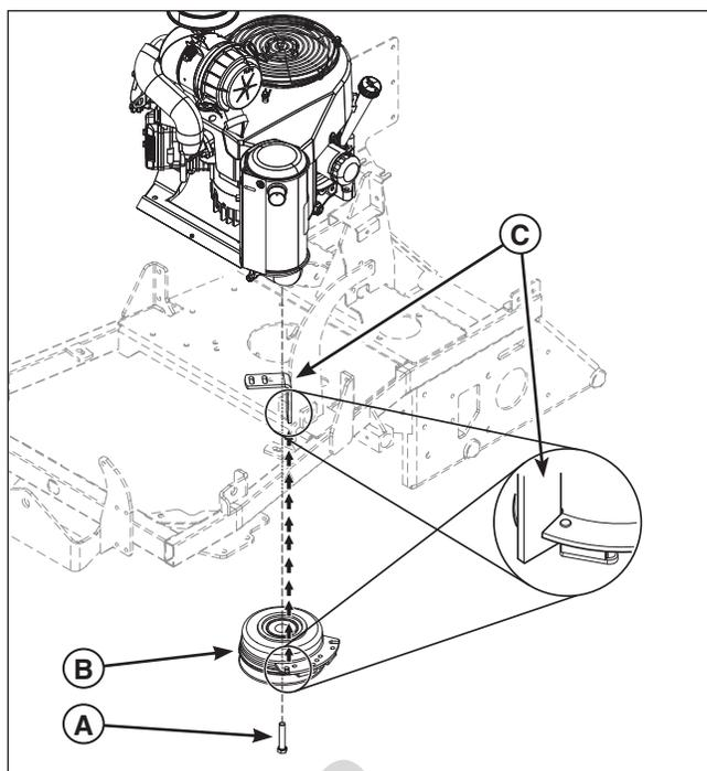
Figure 50. Removing the PTO Clutch
