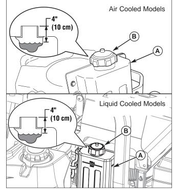
Figure 16. Checking Hydraulic Oil Level A. Hydraulic Oil Reservoir
