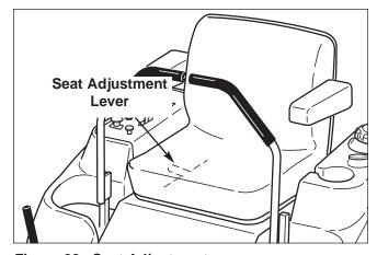
Figure 28. Seat Adjustment
