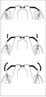
Figure 3. Move Control Levers Gradually
