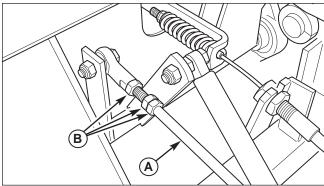
Figure 31. Neutral Adjustment (RH side shown)
