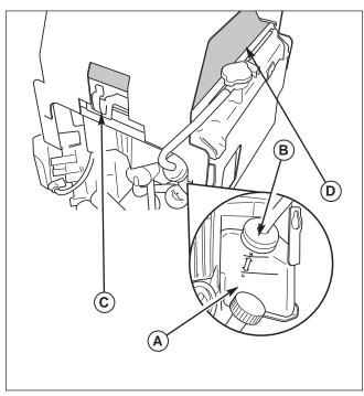
Figure 18. Radiator, Screen & Overflow Bottle
