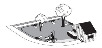
Where possible, make one or two passes around the outside of the area discharging the grass INTO the lawn to keep the cut grass off fences and walks.
