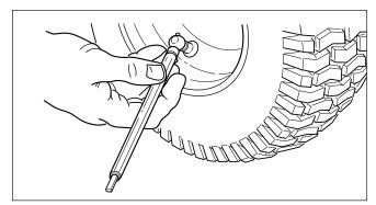
Figure 14. Checking Tire Pressure
