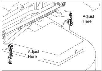
Figure 41. Hanger Chain Adjustment
