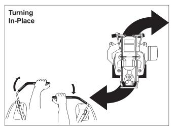
Figure 7. Turning in Place
