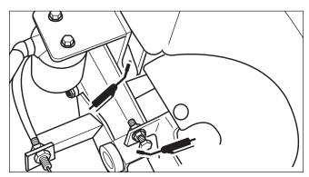
Figure 23. Suspension & Deck Lift Pivots
