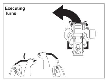
Figure 6. Turning Around a Corner
