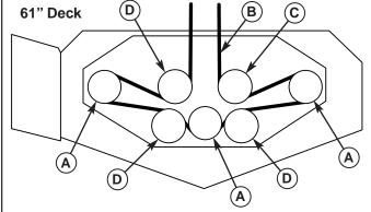
Figure 45. Mower PTO Belt Routing
