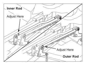
Figure 39. Adjust the Inner & Outer Lift Rods
