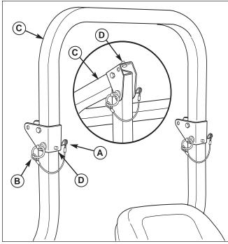
Figure 13. Raise & Lower the Roll Bar
