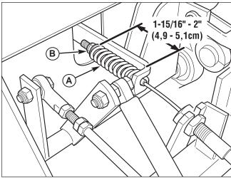
Figure 33. Parking Brake Adjustment
