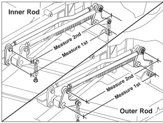
Figure 37. Measure the Inner & Outer Lift Rods
