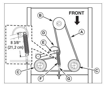
Figure 43. Hydraulic Pump Drive Belt Replacement
