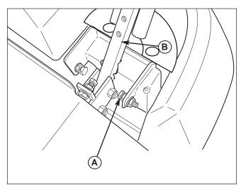
Figure 30. Top Speed Adjustment A. Top Speed Adjustment Bolt
