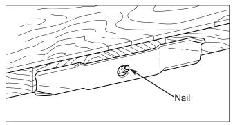
Figure 26. Balancing The Blade
