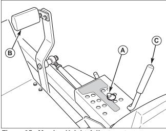
Figure 35. Mowing Height Adjustment
