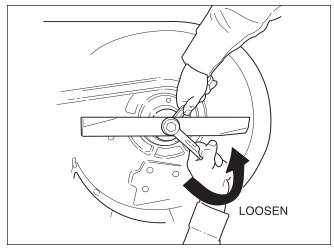
Figure 25. Removing the Blade
