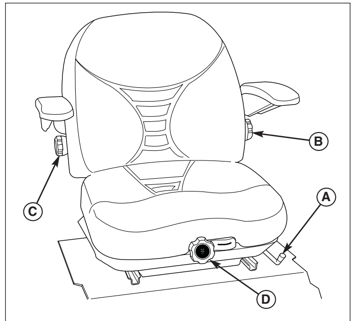
Figure 31. Suspension Seat Adjustment A. Forward / Backward Seat Adjustment Lever B. Lumbar Adjustment Knob C. Back Angle Adjustment Knob D. Suspension Adjustment Knob
