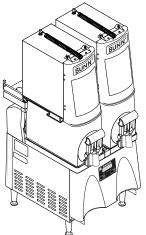
14. Install PAF unit onto platform and plug power cord into rear of platform. Plug platform power cord into proper outlet. (Refer to PAF manual for water connections)(Proceed to step 17)
