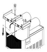
Tighten support rod from top of platform. Retighten motor cover screws.
