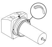
Install each hopper seal over 8. the flange at the rear of the cooling drums as shown.
