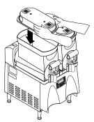
**15.** Set the lids on the hoppers. Lift slightly and slide back or front for filling.
