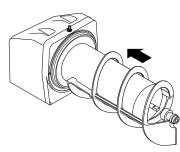
2. Align the auger shafts with the augers. Push the augers as far as they will go and rotate them so the flat face of the auger shaft is aligned with the flat face of the auger nose.
