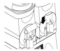
8. Slide the faucet valve assembly into place on the hopper.
