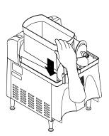
**12.** Slide them into place and push them down until the hopper lock plungers snap into place. For models without PAF, proceed to step 15.
