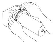
1. Install the seals over the flange at the rear of the cooling drums and press the seals firmly into place as shown.
