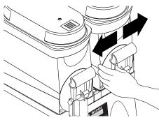
**9.** Press down on the valve to compress the spring. Position the faucet handle over the faucet valve one side at a time and snap into place on the hopper.
