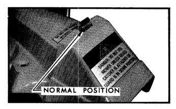
CATCHER POSITION: When using the grass catcher, the deflector must be in the position as shown. The catcher mounting bracket is shown installed, for details showing how to install and use the Yard-Man Grass Catcher see the instruction sheet packed with the catcher.
