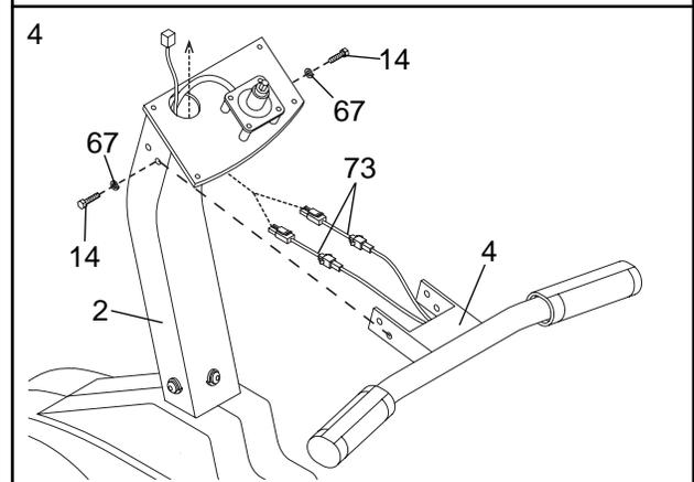
5. Connect the Reed Switch Wire (13) and the two Adapters (73) to the corresponding wires on the Console (8).
