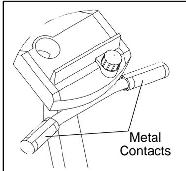
To use the pulse sensor, first make sure that the power is turned on. Stop exercising, rest both feet on the floor, and place your hands on the metal contacts. Your palms must be resting on the inner contacts and your fingers must be touching the outer contacts. Avoid moving your hands. After a moment, the heart indicator in the PULSE display will flash and your heart rate will be shown. For the most accurate heart rate reading, continue to hold the contacts for about 15 seconds.
