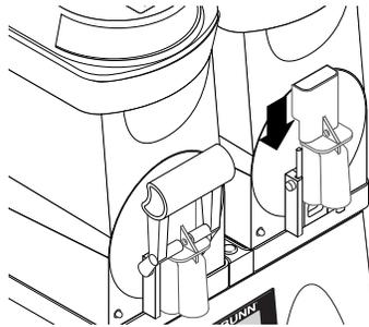
**8.** Slide the faucet valve assembly into place on the hopper.
