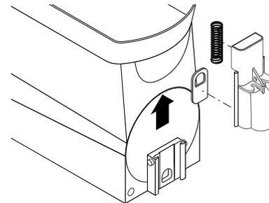
7. Carefully slide the faucet valve up to remove the spring and faucet seal. Extra care should be taken when handling the seal to prevent damage. Do not fold the seal as this will cause damage to the Teflon<sup>®</sup> sealing surface.
