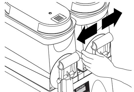
**9.** Press down on the valve to compress the spring. Position the faucet handle over the faucet valve one side at a time and snap into place on the hopper.
