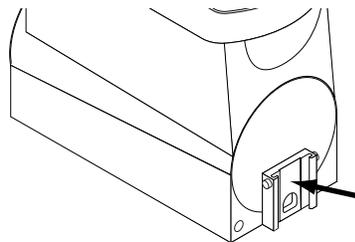
9. Care must be taken to ensure this surface does not get scratched during cleaning. Deep scratches could cause leakage around the seal.
