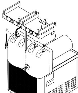
4. Place PAF platform assembly on top of the motor covers and install support rod into hole in trim strip.
