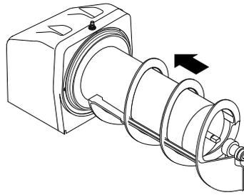
**2.** Align the auger shaft(s) with the auger(s). Push the auger(s) as far as they will go and rotate so the flat face of the auger shaft is aligned with the flat face of the auger nose.
