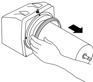
5. Remove the cooling drum seal from the rear of the drum.
