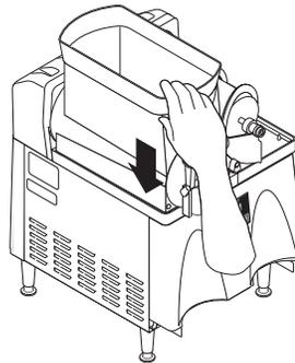
**5.** Slide into place and push down until the hopper lock plunger(s) snap into place. On models with autofill, reconnect fill hoses and level probe to hopper.
