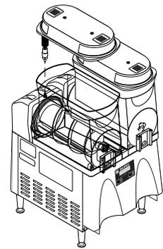
**6.** Set the lids on the hopper(s) and plug in the hopper lid lamp cord(s).
