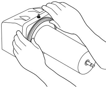
**1.** Install the seal(s) over the flange at the rear of the cooling drum(s) and press the seal(s) firmly into place as shown.
