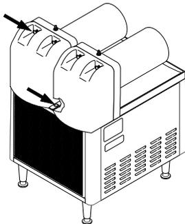
3. Remove the rear plastic plug from the trim strip between the hopper drip trays and loosen the auger motor cover screws.
