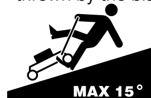
Mow across slopes, not up and down. Do not mow any slope that has an angle of greater than 15°
