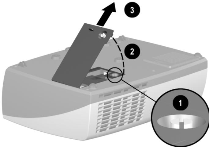
7. Use a coin or flathead screwdriver to remove the two screws from the lamp module ④.
